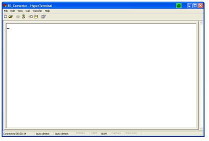
5. Press the " ` " key continuously and then power on the IE-CS(T)-2TX-xRS232/485.
