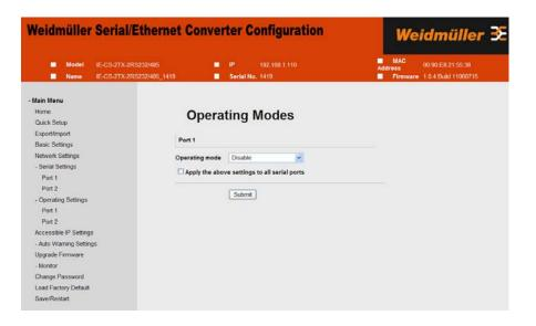
When Operation mode is set to Disabled, that particular port will be disabled. Check the "Apply the above settings to all serial ports" to apply this setting to the other port.
