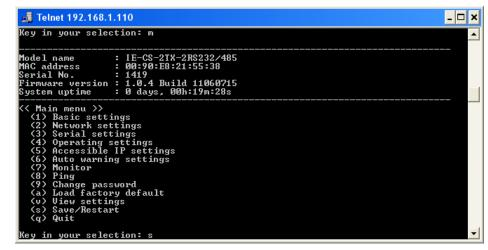
10. Type y and then press Enter to save the new IP address and restart the IE-CS(T)-2TX-xRS232/485.
