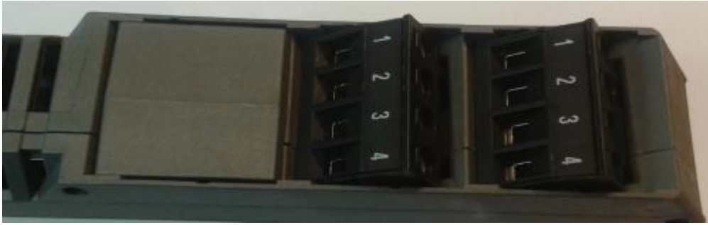
Figure 7 - Terminals on the top side, with cover over the switch.
