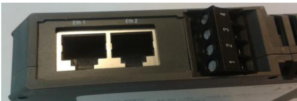
Figure 11 – Bottom side terminal connections.
