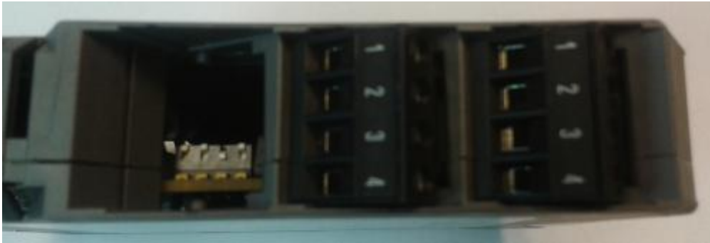
Figure 8 - Terminals on the top side, with cover removed and switch accessible.
