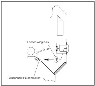
Fig. 80: Remove the cover (2)
