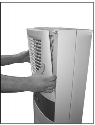
Fig. 35: Remove the top louvred grille
