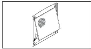
Fig. 26: Installing the filter mat
