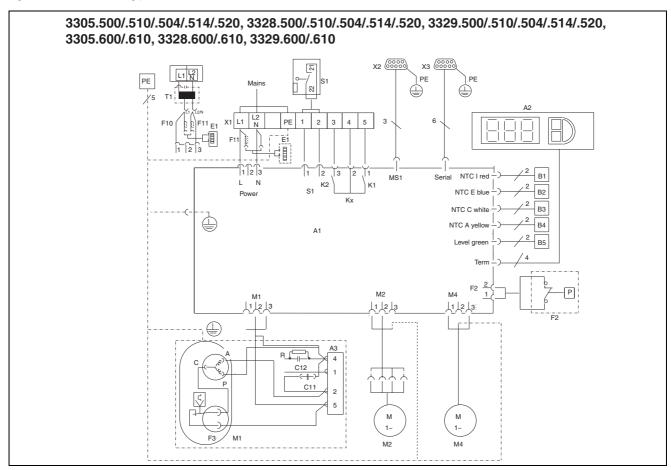
Fig. 115: Electrical wiring plan no. 5
