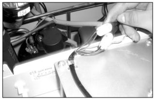
Fig. 66: Disconnect the fan connectors (2)
