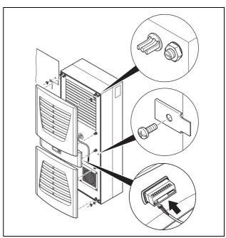
Fig. 18: Securing the cooling unit
