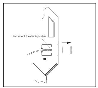
Fig. 81: Remove the cover (3)
