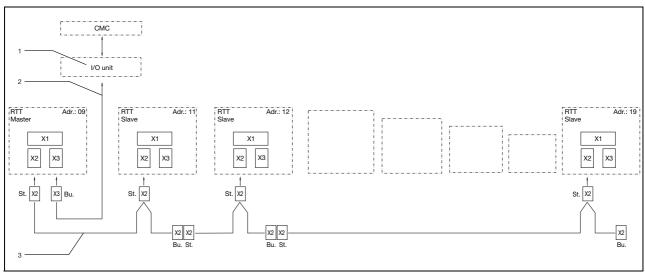
Fig. 21: Connection example: Master-slave operation
