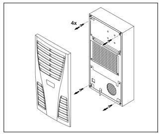
Fig. 17: 3302.xxx only: removing the four screws
