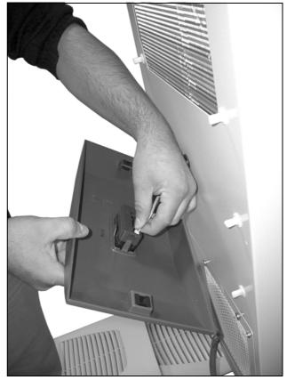
Fig. 38: Disconnect the connector from the display (1)
