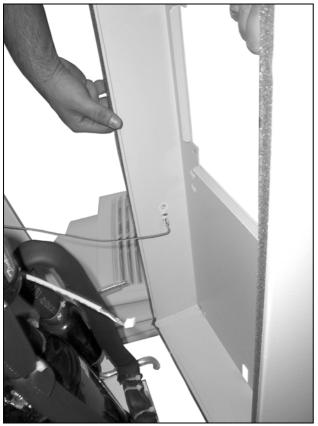
Fig. 72: Disconnect the earthing cable (1)
