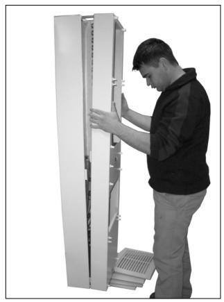
Fig. 71: Removing the cover
