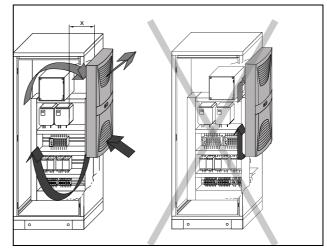
Fig. 5: Air circulation inside the enclosure
