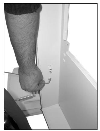
Fig. 73: Disconnect the earthing cable (2)
