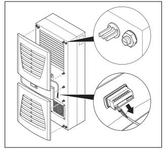
Fig. 10: Removing the louvred grille & disconnecting the display
