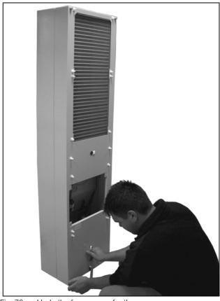
Fig. 70: Undo the four screws for the cover
