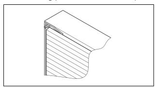
Fig. 12: Applying the self-adhesive tape
