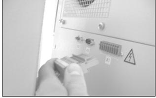
Fig. 34: Disconnect the mains plug
