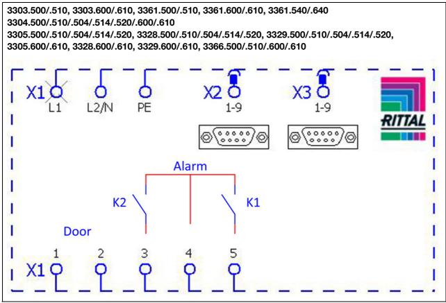
Fig. 24: Electrical wiring plan no. 2
