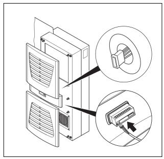
Fig. 14: Connecting the display connector
