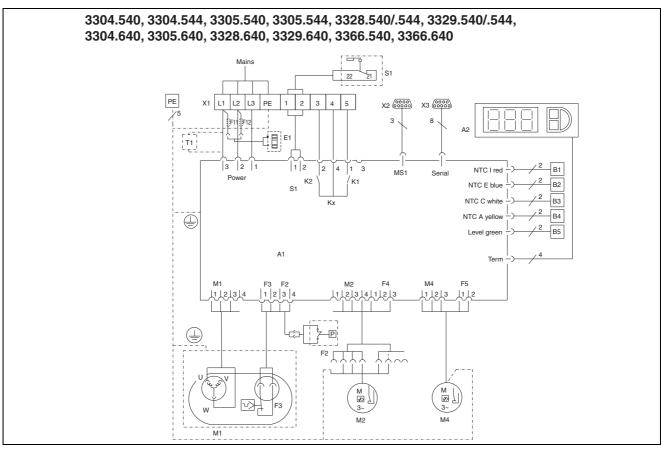
Fig. 116: Electrical wiring plan no. 6
