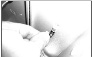
Fig. 69: Disconnect the fan earthing cable (2)
