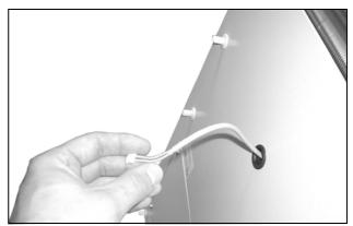
Fig. 45: Slide the display cable back
